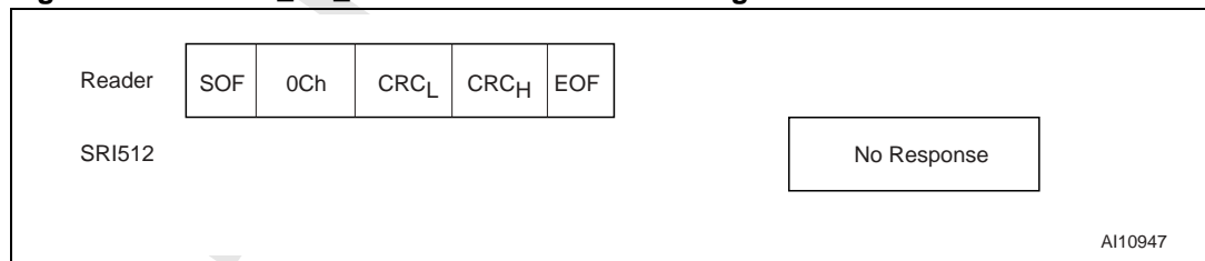
Figure 41. RESET_TO_INVENTORY Frame Exchange Between Reader and SRI512
