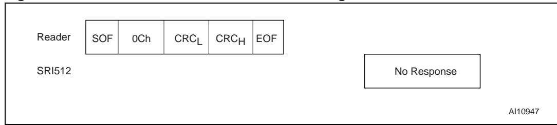
Figure 62. READ_BLOCK Frame Exchange Between Reader and SRI512
